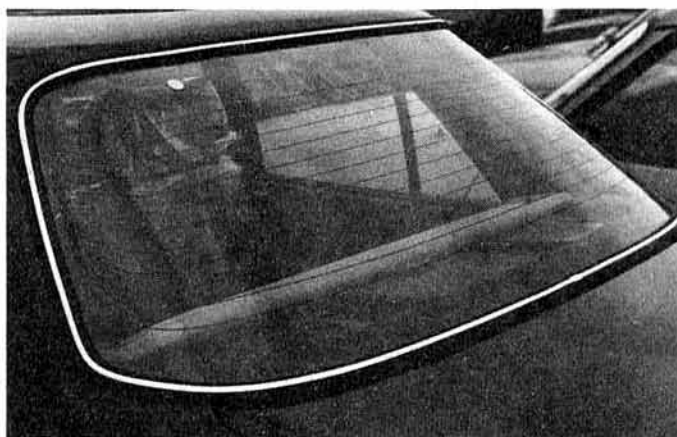
Photo 1. The Ford Orion is one of a range of production cars which use the rear-window heating element as a radio receiving antenna. Both heater terminals are at the same side of the window. They are connected, via an isolator unit mounted in the adjacent roof pillar, to the heater supply and radio
